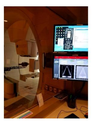
Pencil Beam Scanning paints each proton beam energy layer using fiducials for image guidance while the XRV-124 captures images to memory.
