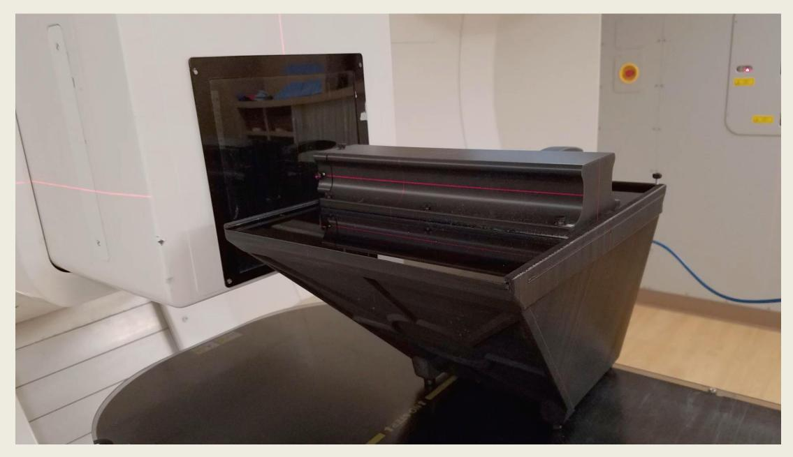
Protons exit the Mevion snout and enter the Ranger scintillator block through a build-up and opaque plastic window
