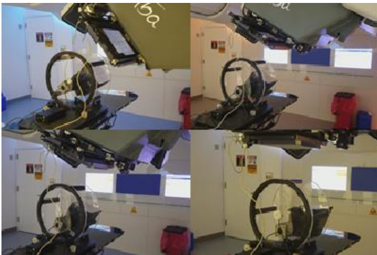
XRV-2000 Falcon mounted in the Motorized Gantry Cradle, automatically following the delivery gantry
