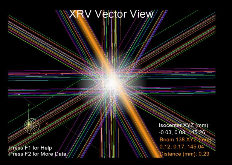
The XRV-124/100 camera phantoms and software automatically map the proton beam isocenter as the gantry rotates.
