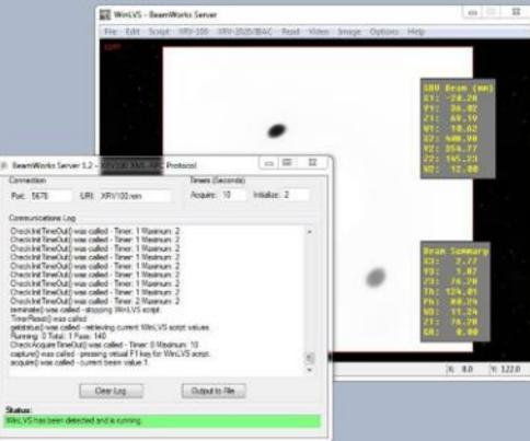
After integration, the treatment system acts as the Client and queries the XRV-124 Server over the Local Area Network using the XML-RPC protocol.
