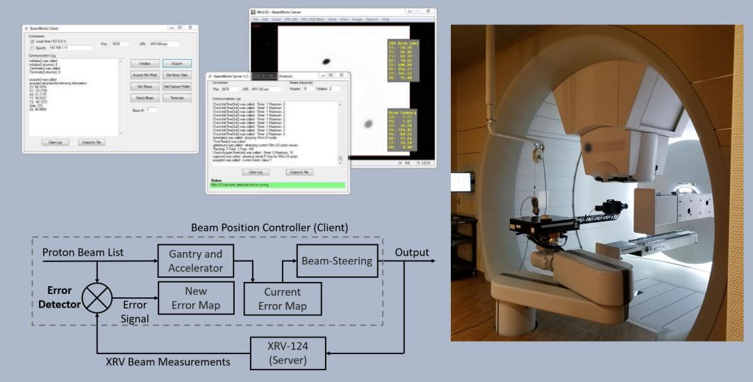
These error maps provide the added precision needed by the proton delivery system to fine-tune treatment plans for the highest possible accuracy.
