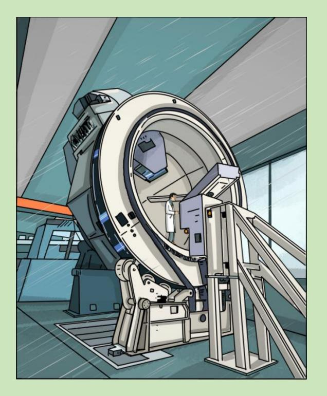
Proton therapy systems are large, heavy, and complex. The gantry, accelerator, degrader, robotic couch, beam-steering magnets, KV imagers, X-ray sources, lasers, and various other elements must be orchestrated precisely to deliver dose to a millimeter-scale target.
