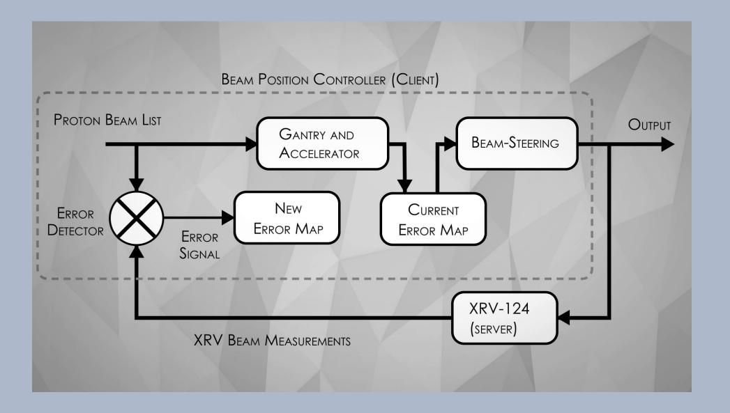
Using the BeamWorks Client-Server, measurements can be automatically fed back into the treatment system to iteratively tune the beam with minimal human interference.
