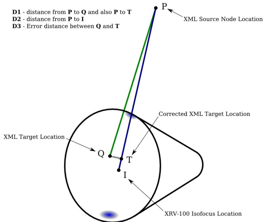
**Figure 6 – Delivery Error Distance Calculation**
