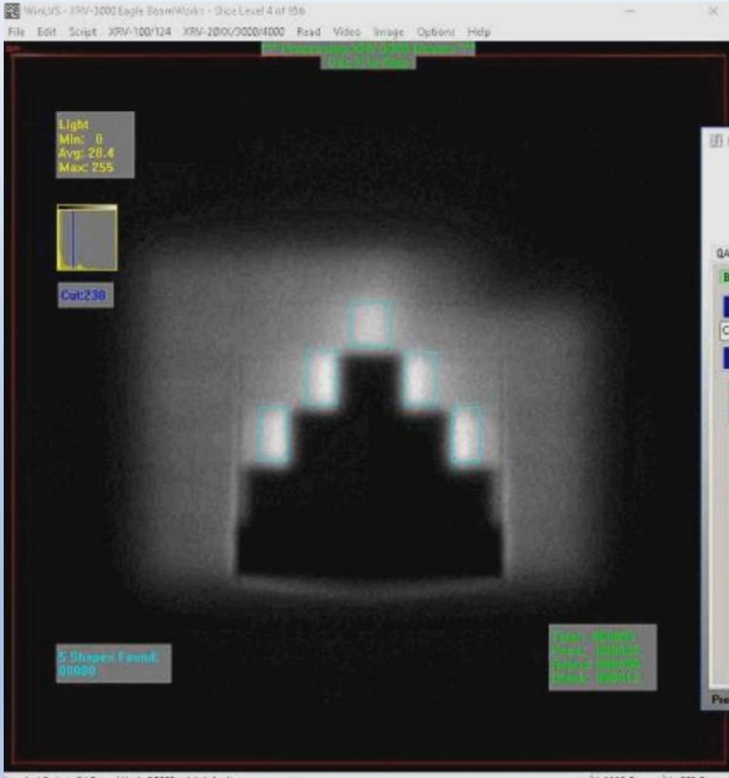
Pressing the Option 1 button starts the process of detecting Bragg Peak regions in the captured images and writing peak-to-peak measurements to file in a CSV format that can be easily imported into the template spreadsheet for analysis.
