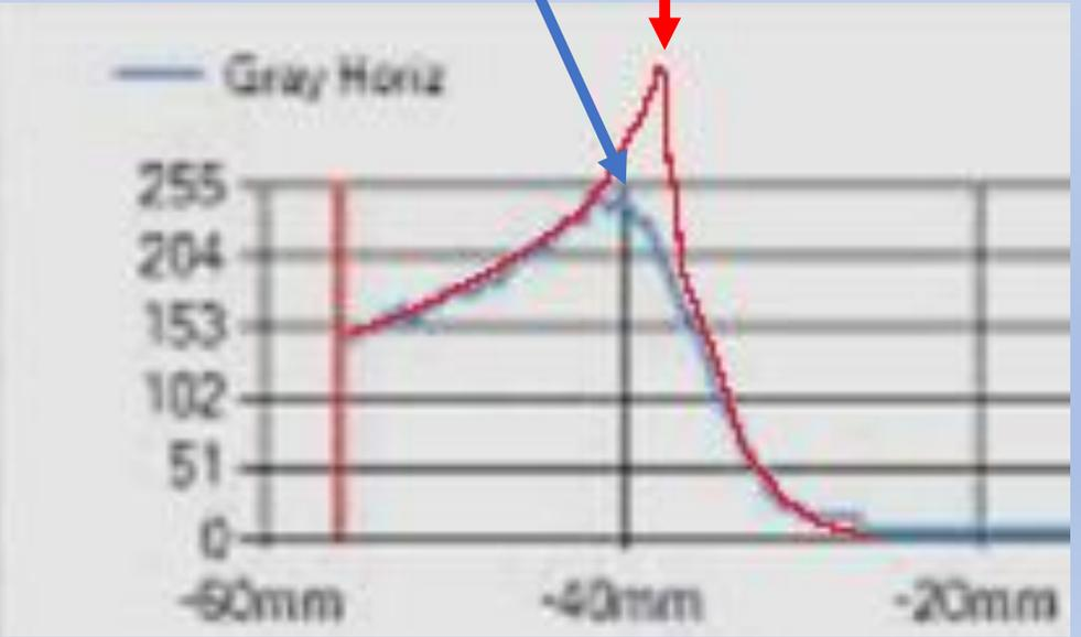
The pristine Bragg Peaks are “quenched” in the scintillator causing the peak-to-peak measurements to be skewed in the proximal direction.
