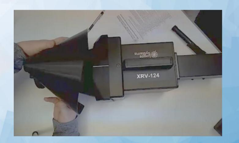
The shroud may be removed during beam capture if the lights and lasers in the treatment room are turned off
