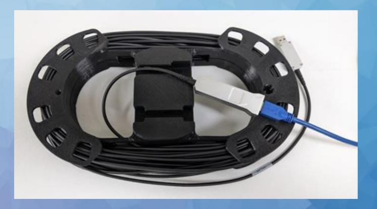
The power-over-fiber-optic cable connects the USB3 cable from the XRV-124 phantom to the laptop or PC USB3 port
