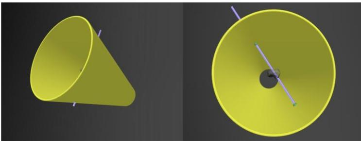
Shown above is a representation of X-ray beams striking the XRV-100 scintillator cone from various angles. Once the entrance and exit spots for each beam are measured, the 3D path can be precisely calculated and displayed in the Vector Viewer application below.
