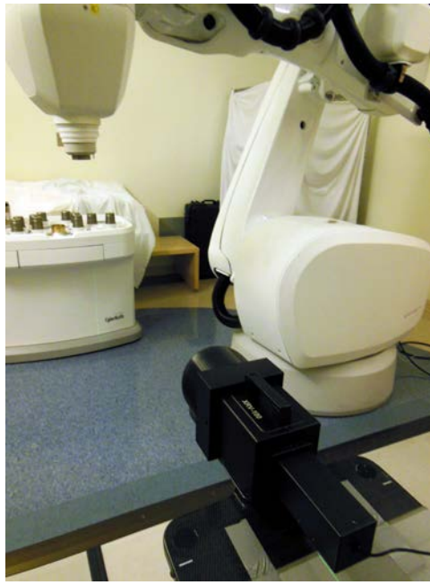
Figure 4—The XRV-100 phantom placed on the treatment couch
