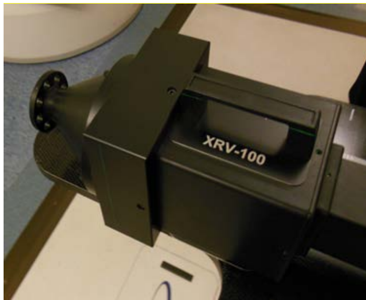
Fig. 1 – XRV-100 phantom with imaging cone shroud removed
