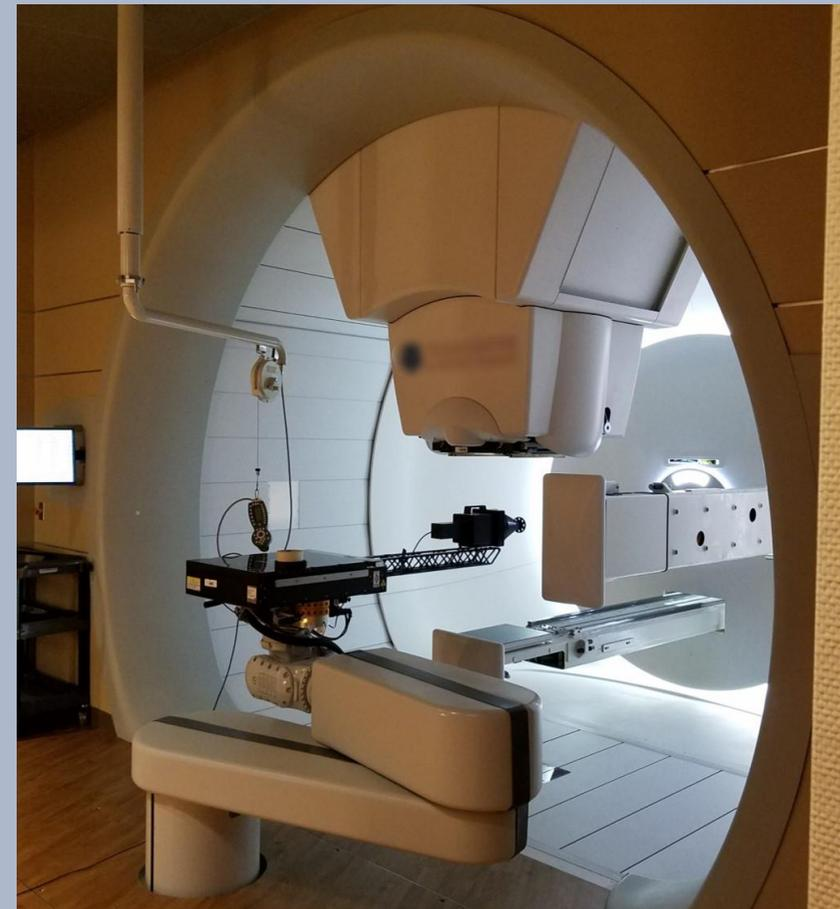
The XRV-124 is best used to create error maps which correct for variations in the gantry isocenter.
