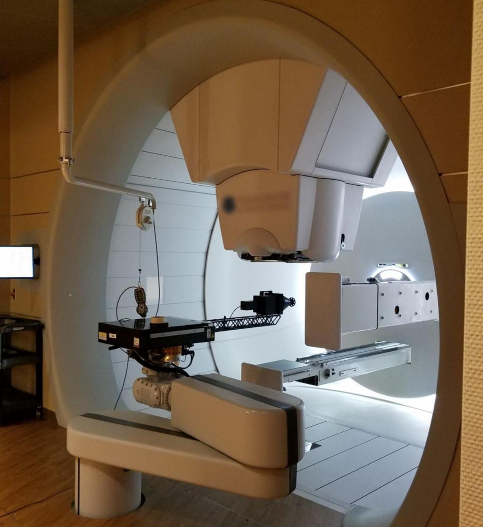
AAPM Task Group 142 guidelines suggest that the radiation beam isocenter should be verified to a 1-mm accuracy on a daily basis for stereotactic radiation therapy.
