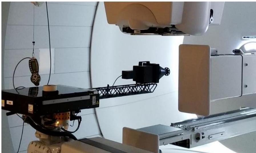
**XRV-124 positioned for closed loop QA with Client-Server**
