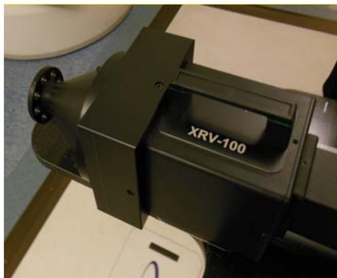
Fig. 1 – XRV-100 phantom with imaging cone shroud removed
