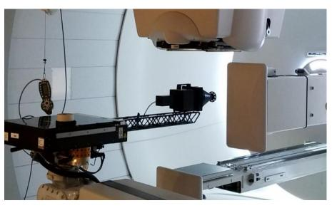
XRV-124 positioned for closed loop QA with Client-Server
